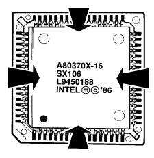
If the coprocessor does not go in smoothly, do not force it; pull it all the way out and try again, keeping it straight as you insert it.
